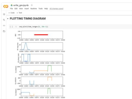
**Figure 4. Pulse timing diagram of the 2D Gradient Recalled Echo sequence.** For clarity, only the first 20 milliseconds of the pulse timing diagram was visualized.
